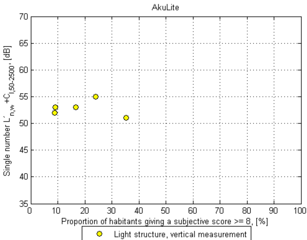
Figures 5a – 5c. The impact sound insulation L'_{n,w} + C_{1,50-2500} plotted versus different subjective ratings, according to question 5.
